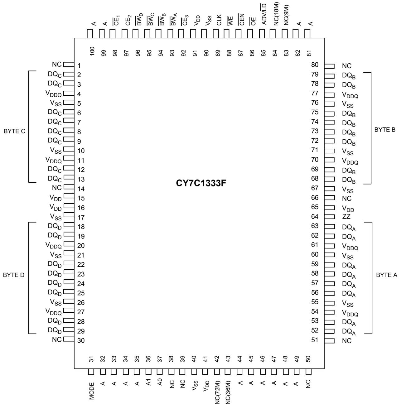
**Pin Definitions** (100-pin TQFP Package)
